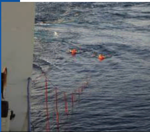
Tori lines deployed on South African Trawler; Keith Davis
